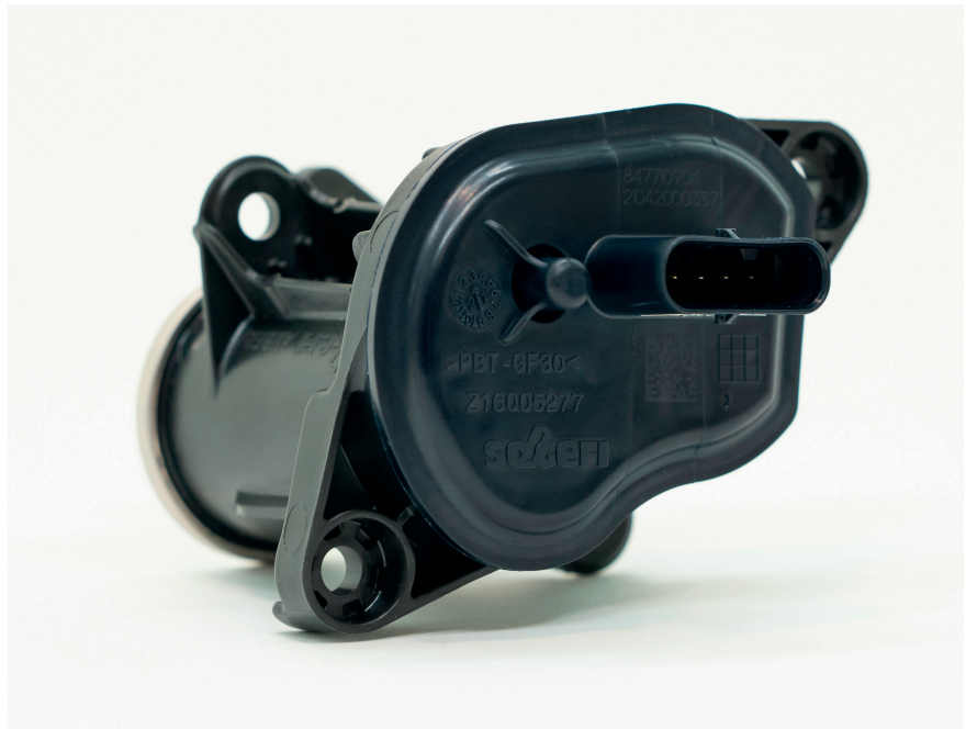
Fig. 4. The lid of the actuator housing is made of Pocan B3233HRLT, which is pigmented in laser-transparent black, while the laser-absorbing half of the housing is made of Pocan B3233HR.
